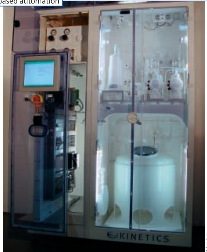
Kinetics chemical distribution cabinet with Simatic WinAC MP
